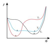
Fig. 1. Changing the order parameter modifies the free energy. Changing the temperature modifies the free energy, F, plotted as a function of an order parameter,  $\Phi$ . The modification of the free energy causes a transition of the system (represented as small circles) from phase A (red curve,  $T_1$ ), first into a mixture A-B phases (blue curve,  $T_2$ ) and then to phase B (black curve,  $T_3$ ). The order parameter could be pressure, density, magnetisation, etc.
