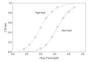
Fig. 10. The motor's response curve, using the non-equilibrium conformation spread model. The motor's response curve (CW bias versus CheY-P level) at zero and high loads, simulated using the non-equilibrium conformation spread model [71].
