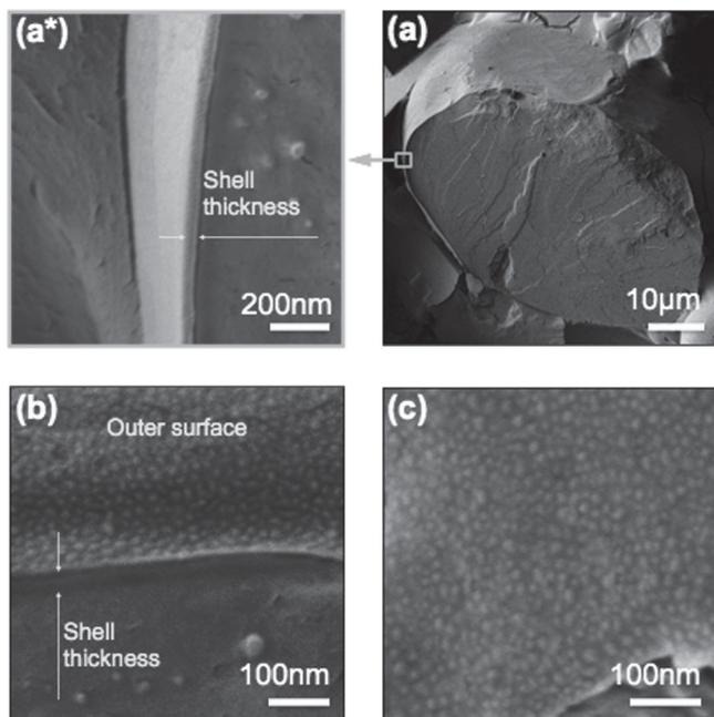
**Figure 2.** Freeze-fracture cryo-scanning electron microscope (cryo-SEM) images of the colloidosome: a) a fractured colloidosome with a highly magnified view of the region in blue shown in panel (a\*), b) the cross-section and outer surface of a thin shell, and c) the outer surface of the shell consisted of densely packed nanoparticles.
