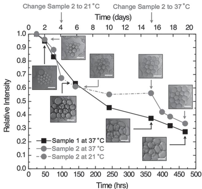
**Figure 3.** Attenuation of the fluorescence intensity in the two samples, each consisting of multiple colloidosomes, at different temperatures, measured using confocal microscopy. The insets are combinations of the fluorescence and bright-field images, in which the scale bars are 200 μm.
