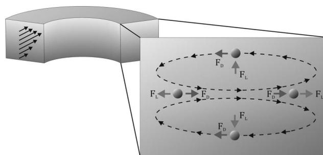
**Fig. 1** Schematic illustration of a continuous curved rectangular microchannel in which both the Dean force ( $F_D$ ) and lift force ( $F_L$ ) are present as well as the directions of their applied force on the particles, resulting in a single equilibrium position at the inner wall of the microchannel, where both forces operate in opposite directions.
