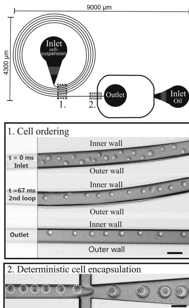
**Fig. 2** Schematic drawing of the microfluidic chip consisting of a curved microchannel followed by an encapsulation part. The pictures are of the cell ordering and subsequent encapsulation. Scale bars are 50 μm.
