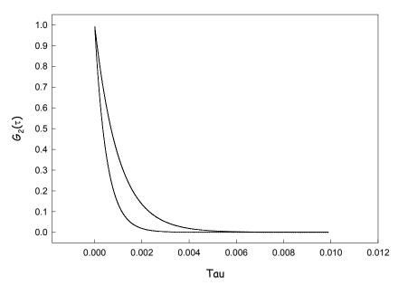
large particles diffuse slower than small particles, and the correlation function decays at a slower rate.
